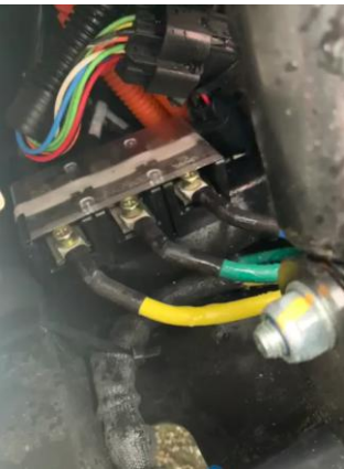
Water get inside after cutting phase wire shield
